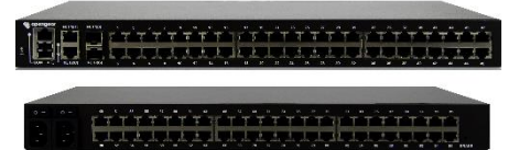
CM7196A – Serials ports on front & back panels
