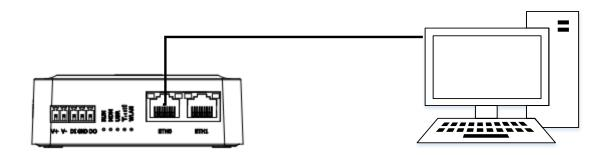
Connect an standard Ethernet cable to the port marked ETH0~ETH1 at the front of the R1510 Router, and connect the other end of the cable to your computer.
