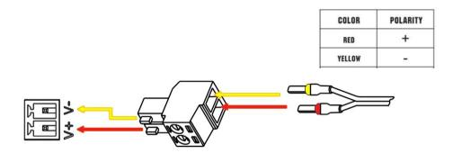
M1200 supports reverse polarity protection, but always refers to the figure above to connect the power adapter correctly. There are two cables associated with the power adapter. Following to the color of the head, connect the cable marked red to the positive pole through a terminal block, and connect the yellow one to the negative in the same way.
