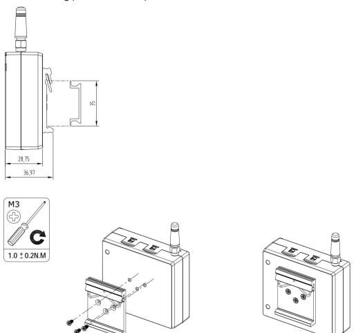
Use 3 pcs of ST3\*8 flat head self-tapping Phillips screws to fix the DIN rail to the gateway, and then hang the DIN rail on the mounting bracket. It is necessary to choose a standard bracket.
