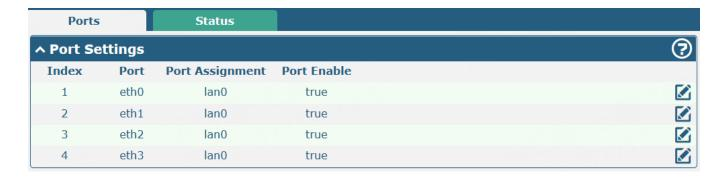
Click M button of eth0 to configure its parameters, and modify the port assignment parameters of eth0 in the pop-up window.
