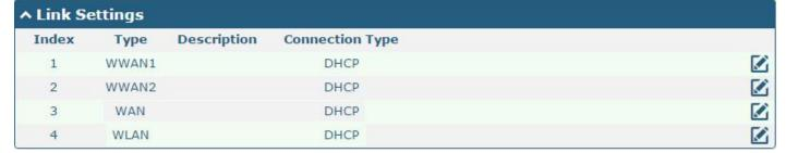
Click the <a> button of WWAN1 to set its parameters according to the current ISP.</a>
