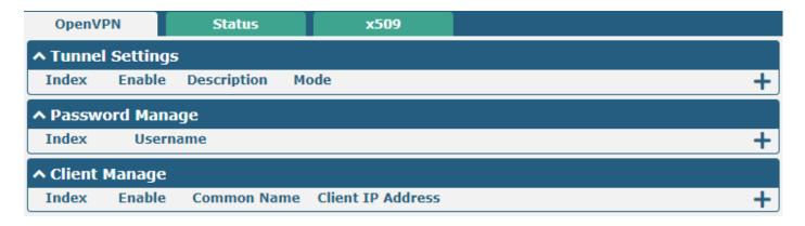
Click to add OpenVPN tunnel settings. The maximum count is **5**. "Mode" is set "P2P" by default. The window is displayed below when choosing "P2P" as the mode.
