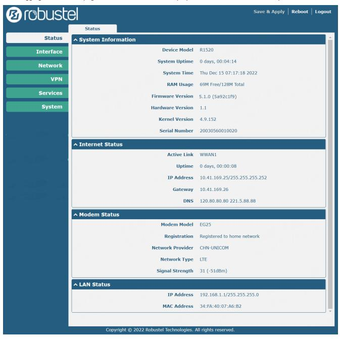
On the homepage, users can perform operations such as saving the configuration, restarting the device, and logging out.
