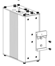
6. Grounding the Device. Grounding will help to prevent the noise effect due to electromagnetic interference (EMI). Connect the device to the site ground wire by the grounding screw before powering on.
